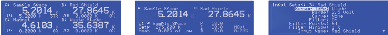
FIGURE 1-2 Displays showing four loop mode, input display mode and custom display mode
