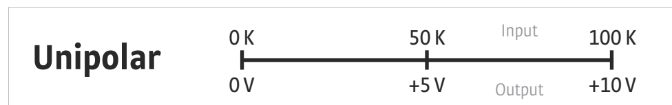
FIGURE 5-4 Output with polarity parameter set to unipolar
