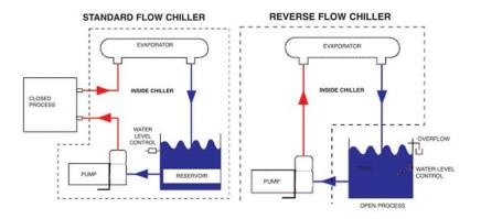
Note - items shown within the dotted borders represent components located inside the chiller.
