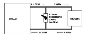
Figure 3.2E Typical low flow by-pass loop
