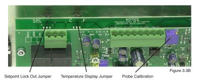
3. SETPOINT LOCK OUT JUMPER: This jumper controls whether the user is allowed to reduce the setpoint below 48°F or 9°C. If the jumper is in position 1 (farthest from the SPL label) the user IS NOT ALLOWED to reduce the
