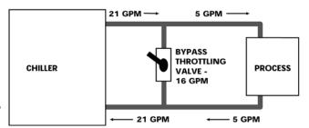
Figure 3.2E Typical low flow by-pass loop
