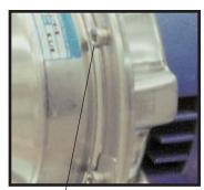
Typical pump casing bolt
