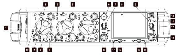
Press the Menu button (**11**) to step back in the Menu. Select number 9, "Quick Setup." Note: Photo shows Daylight option <u>off</u> in menu. Then Select number 1, "Load Settings."
