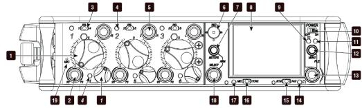
When recording or in playback this switch lets you listen to the isolated channel, but in stop mode, it turns on the Channel Settings menu for the channel it is close to. So toggle the switch to the left and you should see this menu. Notice it says it is CH1.
