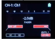
The input impedance type and phantom power, are accessed by pushing the Headphone Encoder knob and rotating until MIC-PH is highlighted in *burnt orange*.
