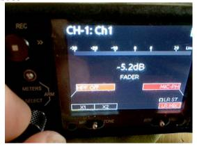
Repeat this for Channels 2 and 3 as needed. If using wireless lavs on 2 and 3, leave phantom power off.
