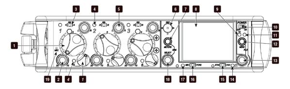
Access the Main Menu by pressing Menu button (12) once. Use the Headphone Encoder knob (13) to highlight number 7, "FILE STORAGE." Push on the Headphone Encoder knob to select. And then turn the Headphone Encoder knob to highlight number 10 "Erase/Format CF." By the way, this white menu is the "Daylight" menu.
