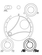
the 80 Hz setting to reduce wind noise and low frequency rumble. The higher settings can be used to counteract the proximity effect of directional microphones where a more gentle slope is desired.
