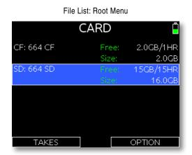
In the Root Menu of the File List, use the Headphone Encoder to highlight either the CF or SD card. Slide the RTN Switch to access options for the highlighted card. Press the Headphone Encoder to display the listing of files and directories on the highlighted card.
