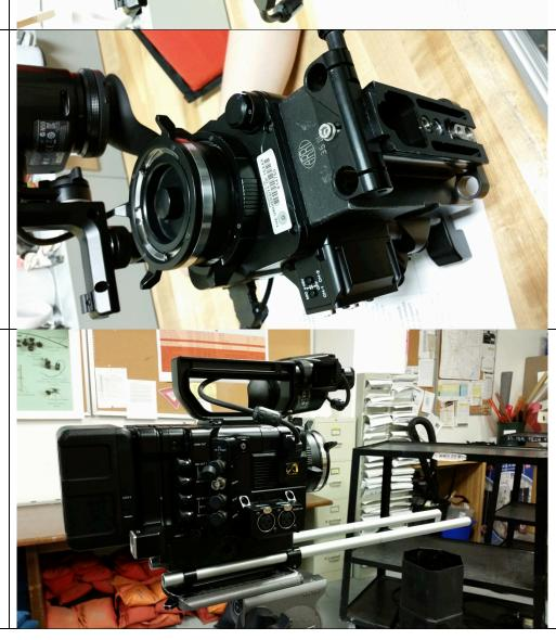
5. Attach the lens to camera and ensure that the PL mount lock is locked. One person should continue to support the lens until the support bracket locked into place!
