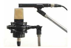
You can also use a single body mic like the Audio Technica BP4029 that has both a bidirectional capsule and a hypercardioid capsule in the same body. In this way you can use this mic on a boom to record dialog using the mid (hypercardioid) mic, but also use the same mic to record stereo in a location, for example for ambiences.
