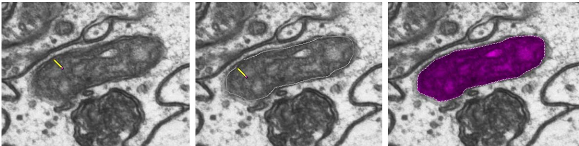
Figure 1.4. Drawing a trace with the freehand drawing tool. (left) Start of the tracing. The pencil is positioned at the profile to be traced and the left mouse button pressed and held down. (middle) Just before release of the mouse button. The pencil left a trail where it was moved with the mouse from the start position. (right) Right after release of the mouse button. The trace is closed and filled with color.
