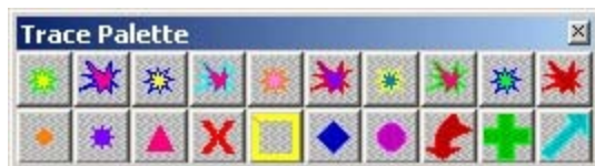
Figure 8.5. The Trace Palette window. The top row of buttons displays the user defined palette entries, while the bottom row displays the predefined palette entries. Each button shows the default border and fill colors, fill style, and Stamp Tool trace shape.
