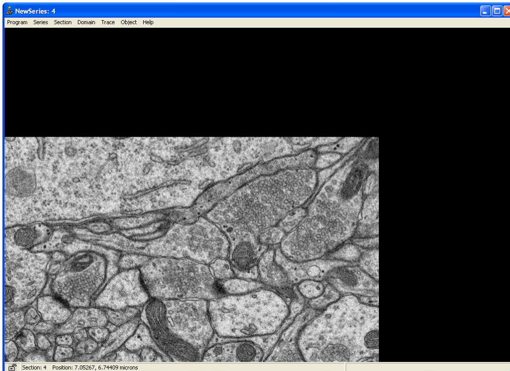
Figure 6.6. A black border may appear around an image. The position of the image relative to the black border is determined by the original transformation used to align the images.
