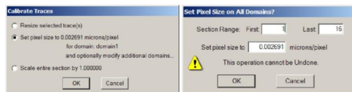
Figure 1.3. The Calibrate dialogs as filled out for a global calibration of the pixel size of images. Top: The first dialog requests that a pixel size calibration be done for the image on which the calibration lines were traced. Bottom: The next dialog allows this same pixel size to be applied to every image in every section of the series.
