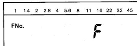
6. Fire the flash unit by pressing its open-flash/test button. The meter will show the f-number reading on its liquid-crystal display.
