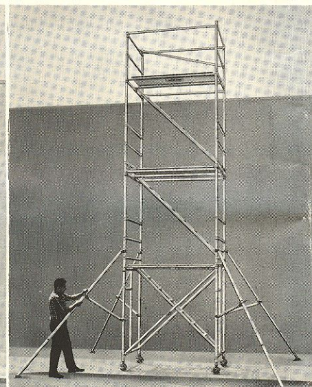
14 Adjustable Outriggers (above, left) or Long Adjustable Outriggers (above, right) may be used instead of outboard supports to provide the necessary base stability. Make sure each outrigger is wedged firmly against solid pavement and all clamps are tightened securely.
