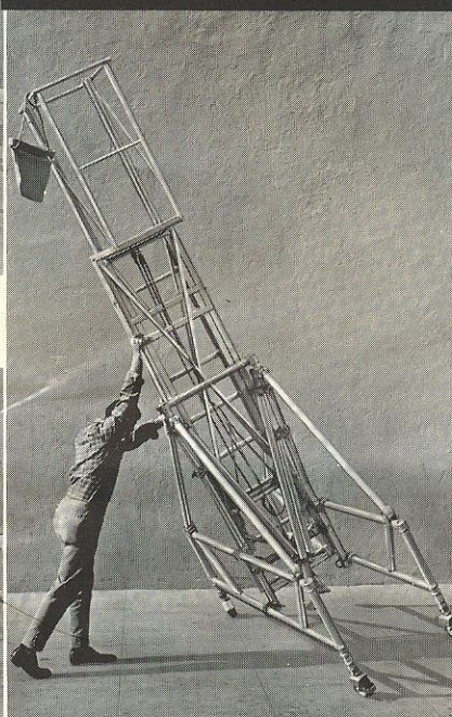
3 Lock the casters and tilt the Tallescope into vertical position.
