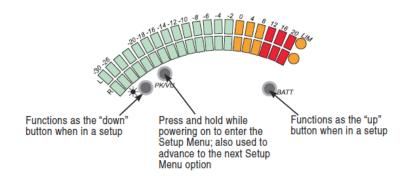
The meter lights will do the "scrolling dance," then the 0dB lights will stay on and the -30dB light for the Left(upper) meter will be blinking. You are now in the set-up menu.
