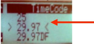
If recording with High Definition Cameras at a 23.976 frame rate set the Time Code Frame Rate to 23.976
