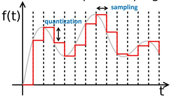
Both lead to "stair step" waveforms
