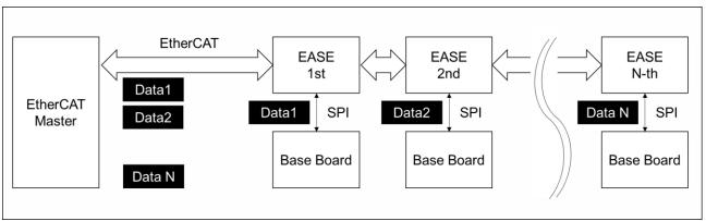
FIGURE 14. DATA FLOW BETWEEN ETHERCAT MASTER, EASE, AND BASE BOARD
