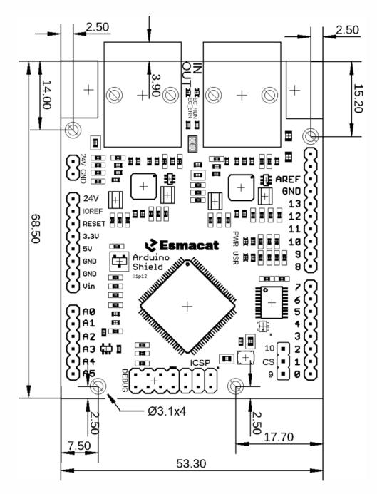
• PCB board height from PCB top layer to the top of RJ45 connector: 14.4mm
