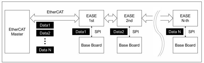
FIGURE 1. DATA FLOW BETWEEN ETHERCAT MASTER, EASE, AND BASE BOARD
