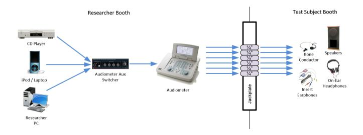
In Booths B & E, the Researcher PC has an 8-channel Mark of the Unicorn (MOTU) 838 USB soundcard. This device is capable of recording up to (2) mic or (8) line sources and playing back up to (8) channels of audio. Outputs 1 & 2 are the primary outputs (aka default Windows playback device) from the computer. These outputs feed to the audiometer via the Audiometer Aux Switcher. Outputs 3 - 8 feed directly to the jackpanel for use in specialized experiments.
