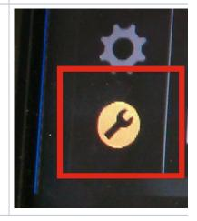
Reset the camera to defaults System Go to System>Scroll down to All Reset press the knob and choose Reset >All Reset>Reset Language **Clock Set** 00:00 **Hours Meter AXS Recorder Basic Authentic** Wi-Fi **All Reset** Option Press Reset again System **⊅** Back Reset Reset>Execute System **⇒** Back Reset Yep Execute again All Reset?
