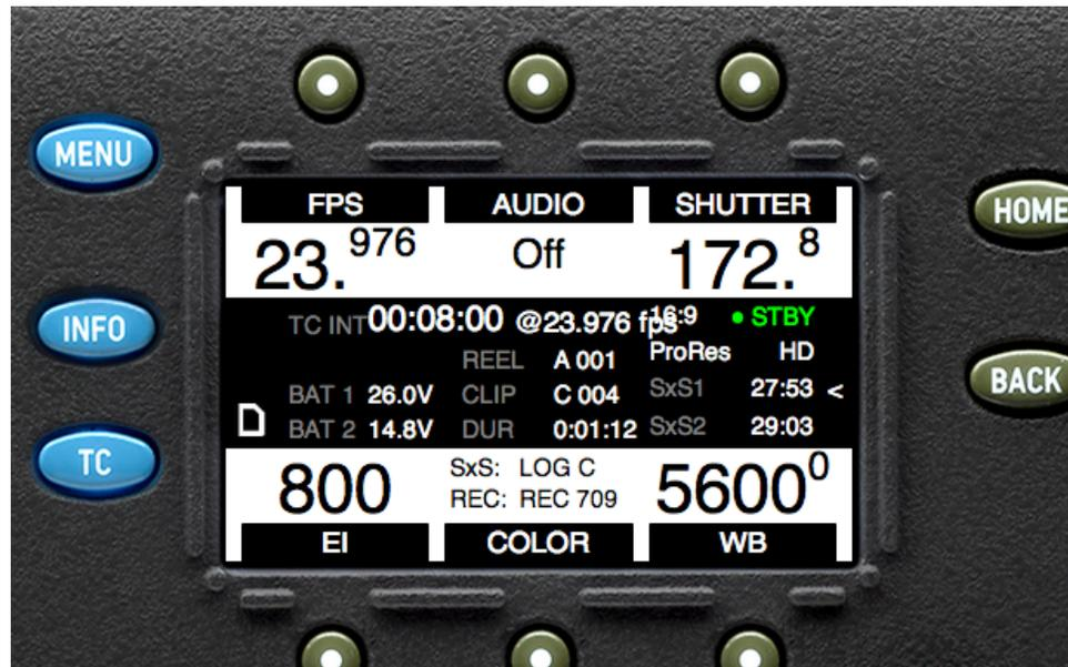
Next change the SXS card recording resolution to 2K. Go to Menu>Recording>Internal >
