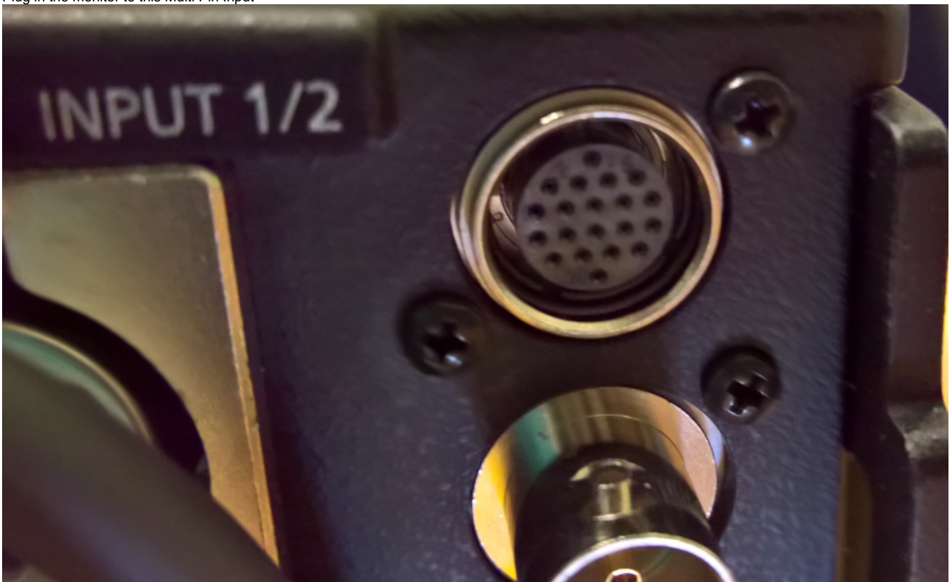
Plug in the monitor to this Multi Pin Input
