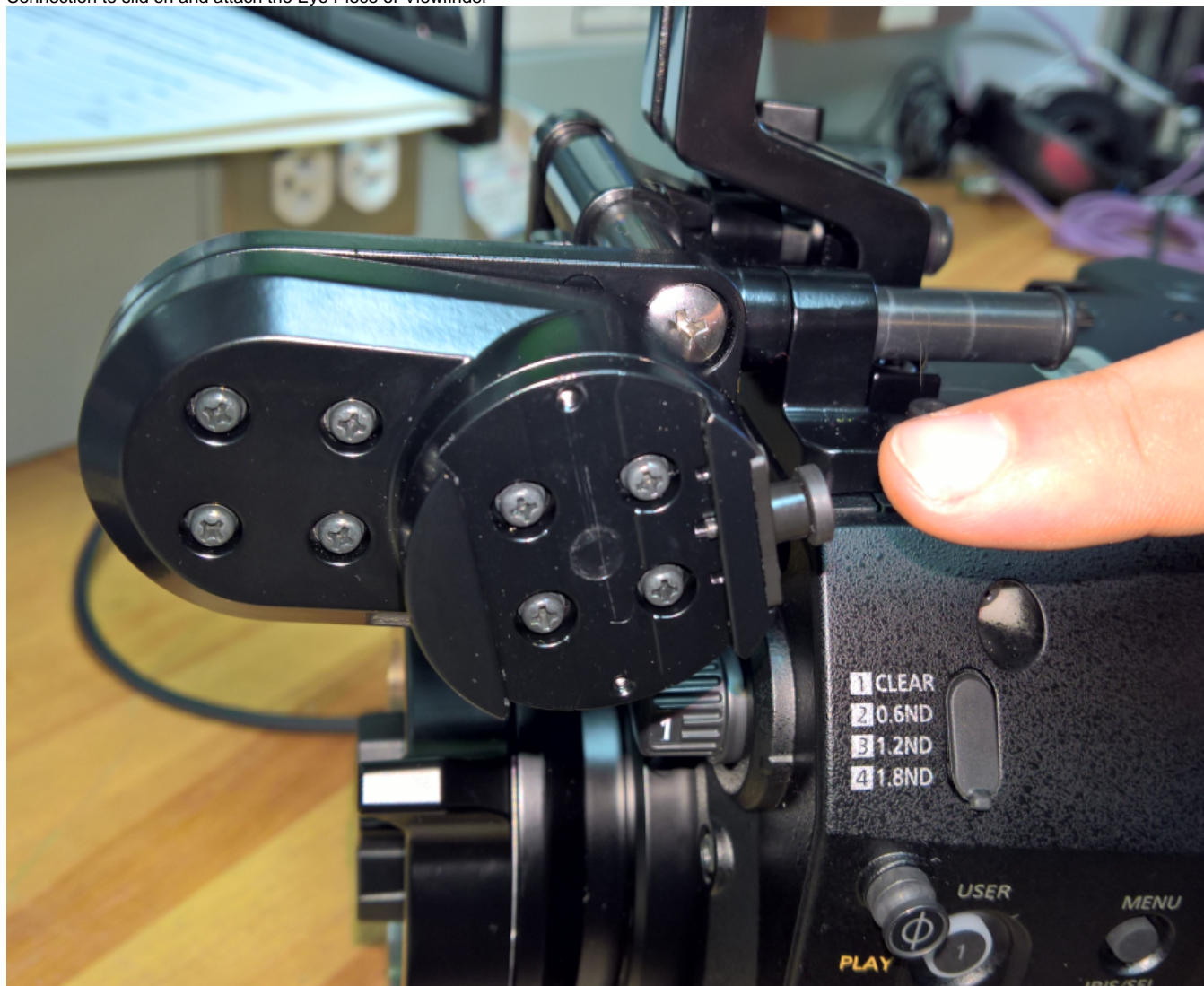
Connection to slid on and attach the Eye Piece or Viewfinder
