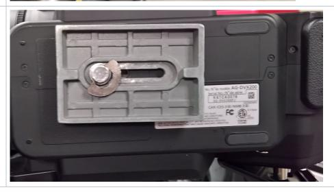
Pull Latch shown here to unlock the plate and push it in to
