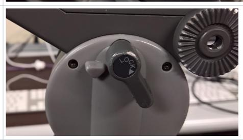
Turn this knob to loosen the pan handle to adjust the position.
