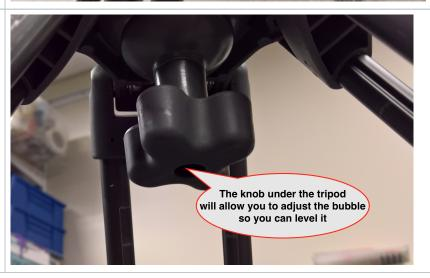
Bubble on the tripod head used to level the tripod
