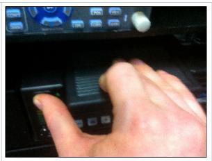
Take the cartridge to DVR1 or DVR2 in 4F Control. Plug the a Firewire 800 cable next to the monitor into the back of the cartridge.
