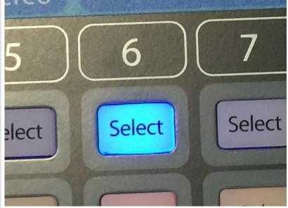
Press Sub 2 and Main to route the audio channel to Sub 2 and Main outputs.
