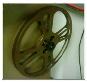
Can and should use split reels for the supply feed reel. Put film on a split reel and put sound mag on a split reel as well.
