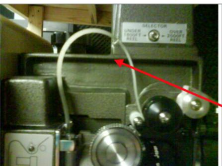
Spool off source reel and thread through the first gate and into the lens gate. Make sure the loop here is as tall as the top of the projector.
