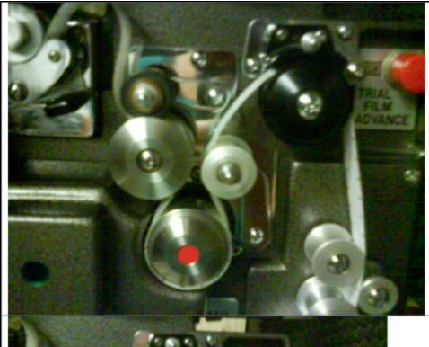
Thread the film as show around these spindles. There are not sprockets on these but there are sprockts on this gate. Make sure it is closed after film is threaded.
