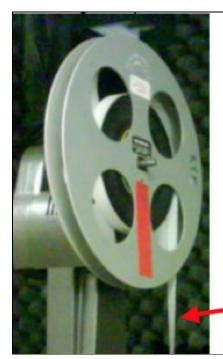
Film needs to be unwinding clockwise with sprockets closest to you when facing the projector. Emulsion (dull) side needs to be on the inside of the unwind. Shiny side out.
