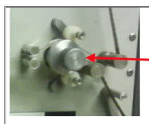
Manual adjustment knob for moving the mag stock manually.
