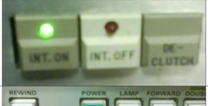
Press INT. ON to turn on Interlock. This will track the movement of the projector and roll the Mag automatically.
