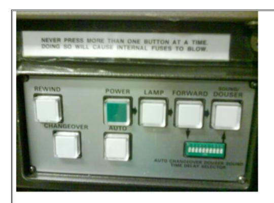
To start film rolling. Press Power then lamp. Light the lamp and then press Forward to start the film rolling forward then open the dowser by pressing the Douser button.
