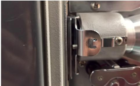
Thread the film through the sprockets following the guide lines in red. Make sure the film sprockets are on the correct side. Only one side of the film has sprockets.
