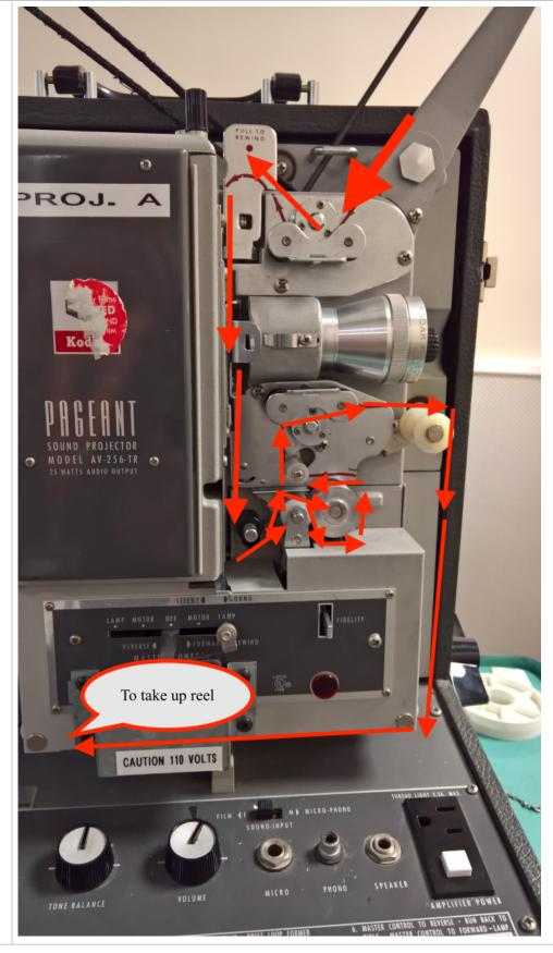
Close up of the lower winding path that is confusing -
