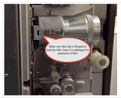
Put in Hinged position (shown here) for the loading of film through the gate
