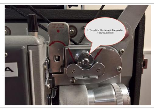
Here is the guide of how to load the film. Follow the red arrows in this diagram as well as the red lined arrows on the projector itself.
