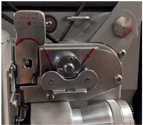
Hinged for the loading of film through the gate and unhinged to hold the film flat on gate for projection playback
