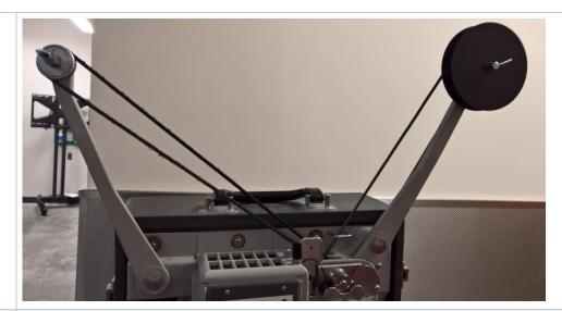
there is a tricky metal flap between the projector arms that needs to be in this up position to load the film.
