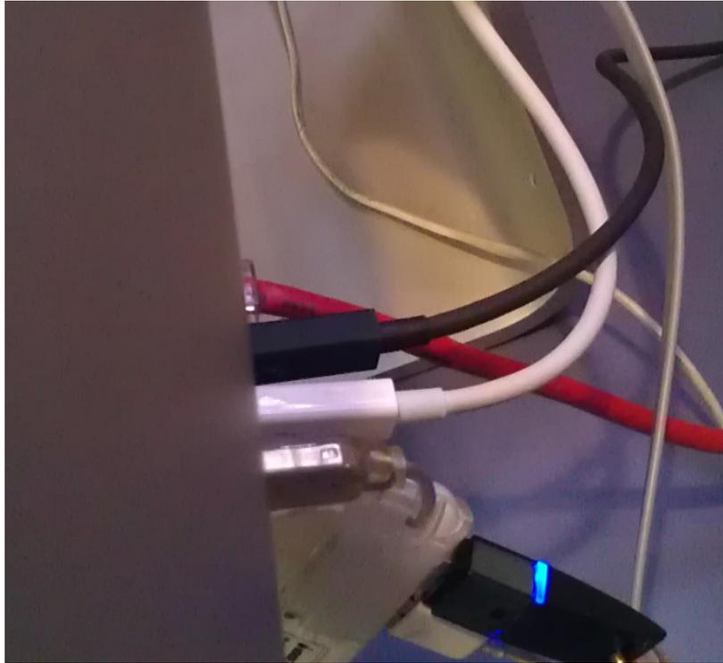
Make sure the other end of the WHITE - Thunderbolt cable is plugged into the Blackmagic Design Intensity Pro as shown here.
