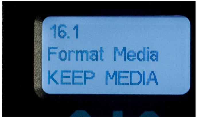
Use the ADJUST up button to select FORMAT. Press the ADJUST up arrow button again. KiPro Mini will display "ERASE S1 [or S2]". Press and hold the ADJUST up arrow button for 2 seconds or longer and then formatting will begin.
