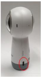
Press the **Power/Back** button for 3 seconds to turn the power on. Note that plugging the camera in will start a battery charging process. You will need to press the power button for 3 seconds to stop that process and turn the camera 'off' before powering up the camera with the power adapter.
