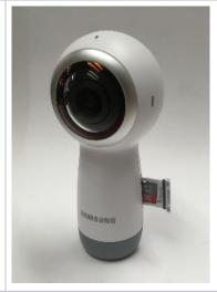
Below the tray is the USB-C data and power port. With a USB power adapter, this camera allows you to keep the camera plugged in while making long recordings.
