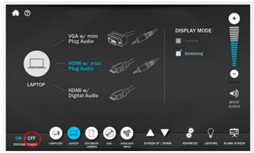
From any screen, press the OFF text in the lower left-hand corner.
