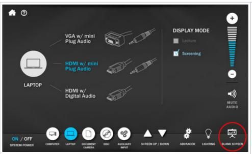
Press the \*BLANK SCREEN \*button at the bottom right to blank the screen. Press it again to restore the picture. Even though the class won't see anything on the screen, you will still be able to see the picture on the teaching console monitor.
