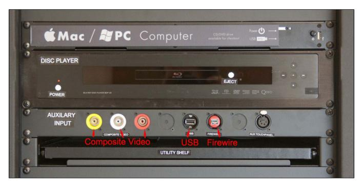
Note the inputs on the left-hand side for composite video and analog audio via RCA jacks.
