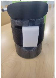
3. On the back of the core Flip the power switch to the 'on' position
