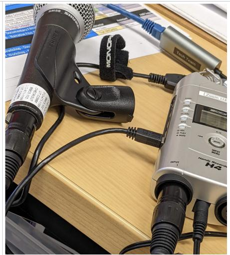
Use the scroll wheel on the side to change the input here to the XLR input you have the mic connecte d in this case it is Input 1
