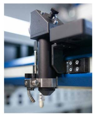
The Air Assist feature on both the Fusion Pro & Fusion Edge Laser is used to keep combustible gases away from the cutting surface and to reduce flare-ups of more flammable materials as you cut through it, such as wood and acrylic.
