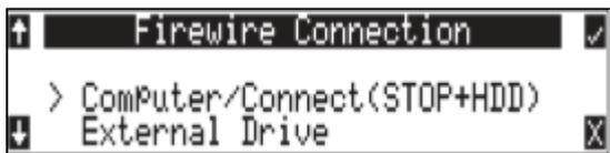
3. Interconnect the unit to a FireWire-enabled computer using an appropriate FireWire cable, as well as any other necessary adapters (ie thunderbolt, usb-c, etc.) No drivers are required if the computer meets the requirements listed in the Specifications. FireWire 400-800 cables are currently provided with all of our Sound Devices digital audio recorders.
