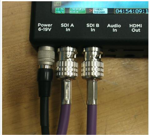
SDI 3 which has the camera menu overlays plug into the monitor input
