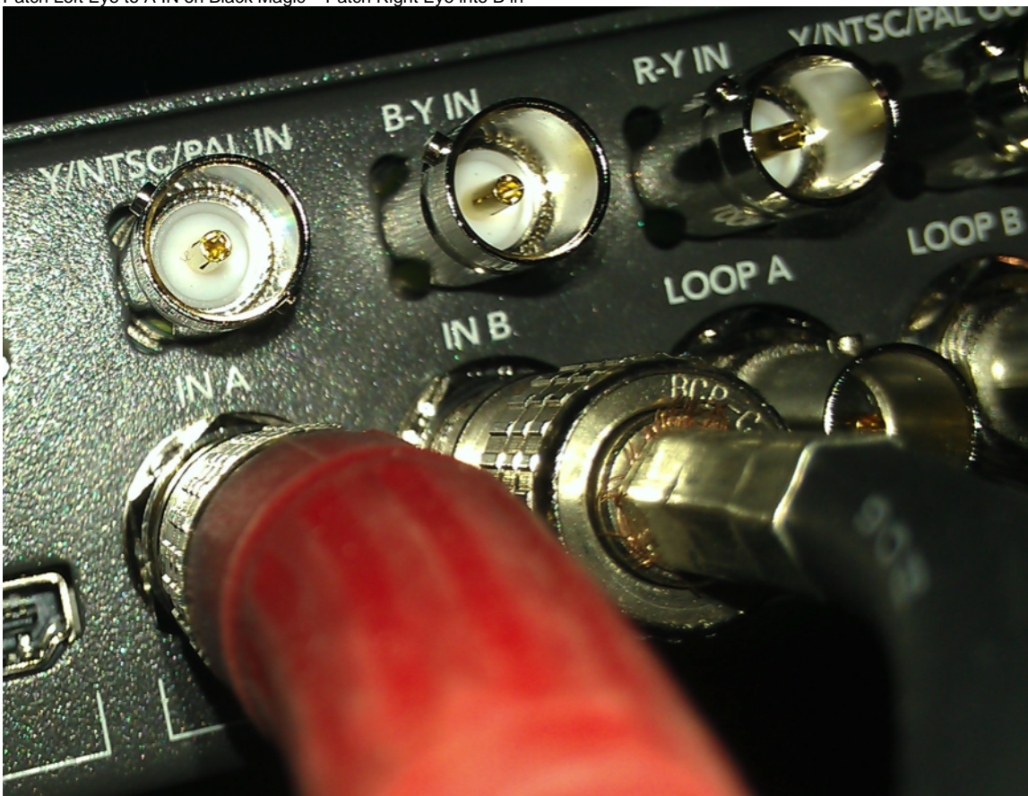
Patch Left Eye to A IN on Black Magic – Patch Right Eye into B in
