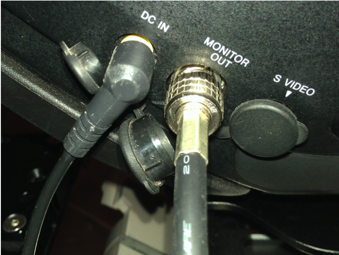
On Left Eye Camera Patch Monitor out to Right Eye Camera Genlock in
